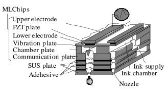
Figure 1: The composition of MLChips type head
